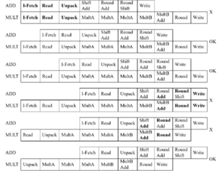
Figure 20.2: If there is only one functional unit of each kind, then an ADD cannot be started at the same time as a MULT (because of numerous resource hazards shown in boldface); nor three cycles after the MULT (because of Add , Round , and Write hazards); nor four cycles later (because of Add and Round hazards). But if there were two adders and two rounding units, then an ADD could be started four cycles after a MULT. Or with dual fetch units, multiple-access register file, and dual unpackers, the MULT and ADD could be started simultaneously.
