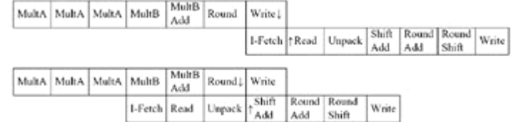
Figure 20.3: Data dependence. (Above) If the MULT produces a result that is an operand to ADD, the MULT must write its result to the register file before the ADD can read it. (Below) Special bypassing circuitry can route the result of MULT directly to the Shift and Add units, skipping the Write, Read, and Unpack stages.
