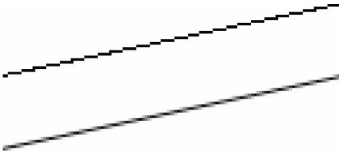
Figure 4.4. On the top we observe aliasing (the stair-step effect when trying to represent a line by a matrix of pixels). On the bottom, we see an antialiased line, which generates the final color of a pixel by sampling and using its neighboring pixels; this results in a smoother image and dilutes the stair-step effect.
