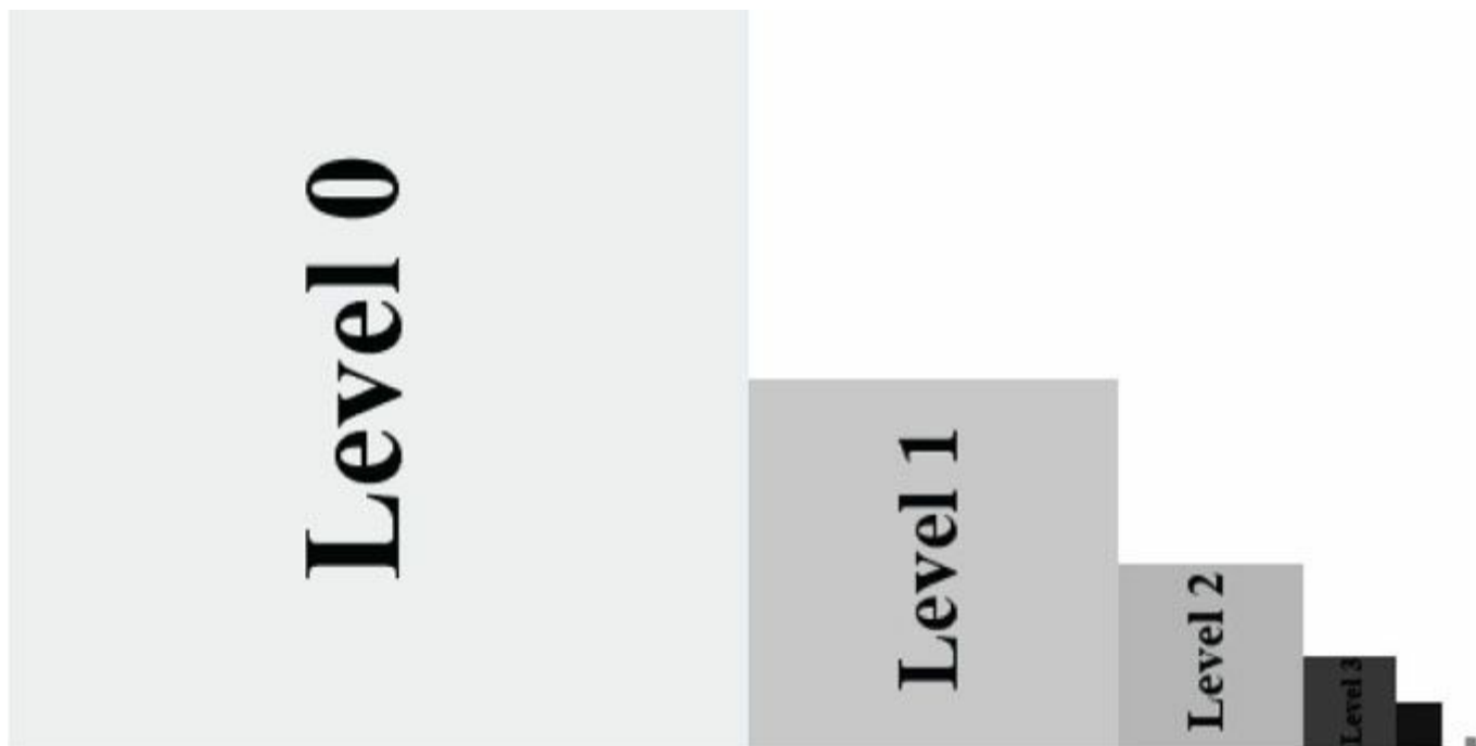
Figure 8.19. A mipmap chain manually constructed so that each level is easily distinguishable.
