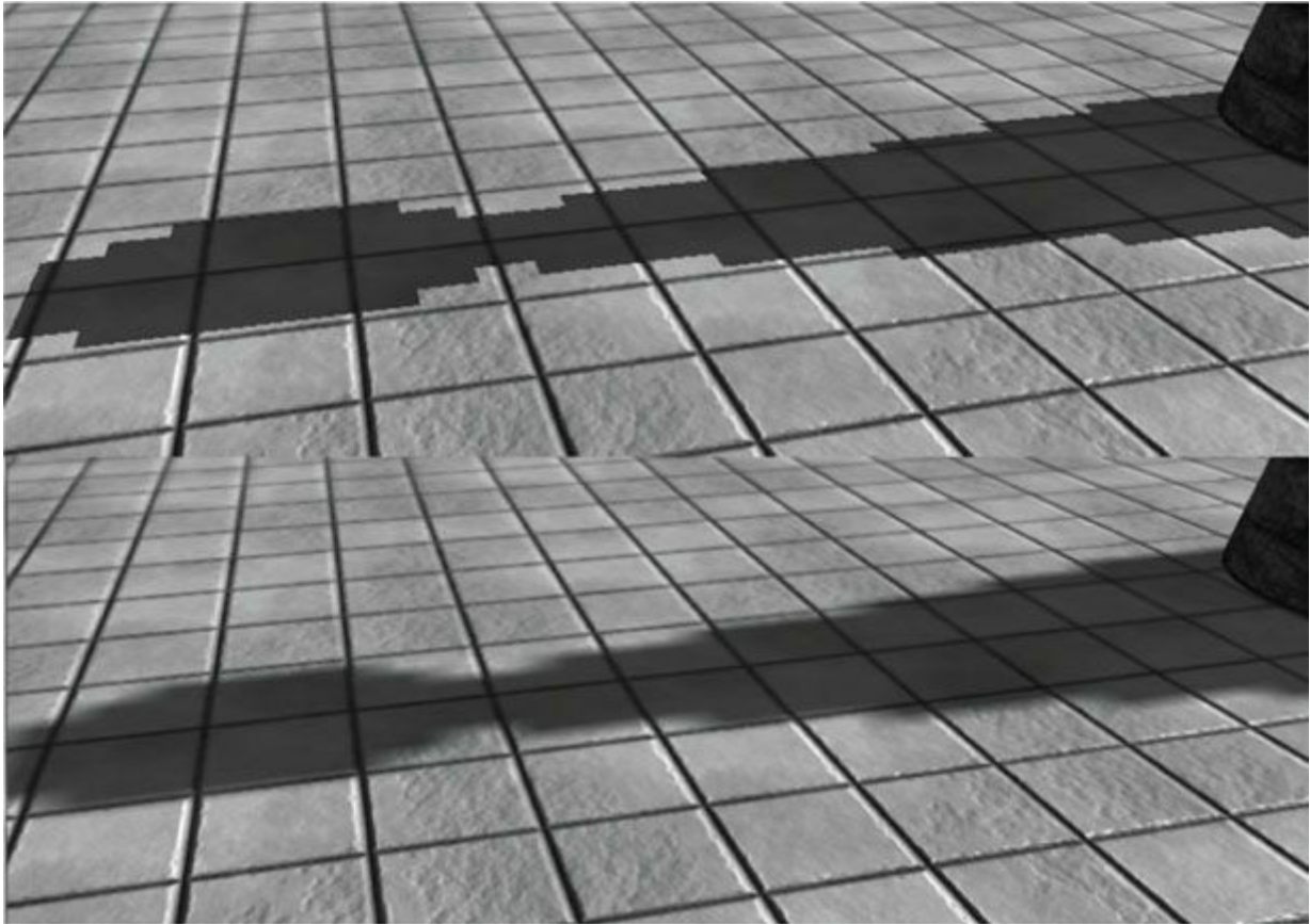
Figure 21.13. In the top image, observe the “stairstepping” artifacts on the shadow boundary. On the bottom image, these aliasing artifacts are smoothed out a bit with filtering.
