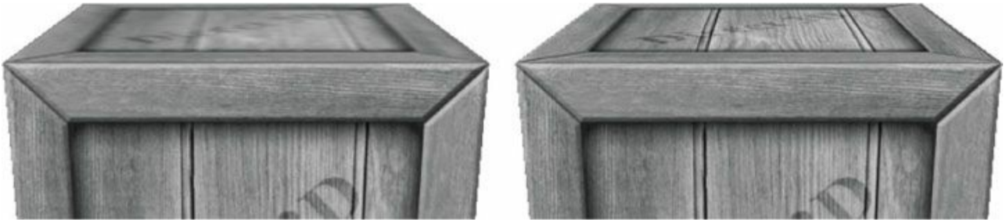
Figure 8.9. The top face of the crate is nearly orthogonal to the view window. (Left) Using linear filtering the top of the crate is badly blurred. (Right) Anisotropic filtering does a better job at rendering the top face of the crate from this angle.
