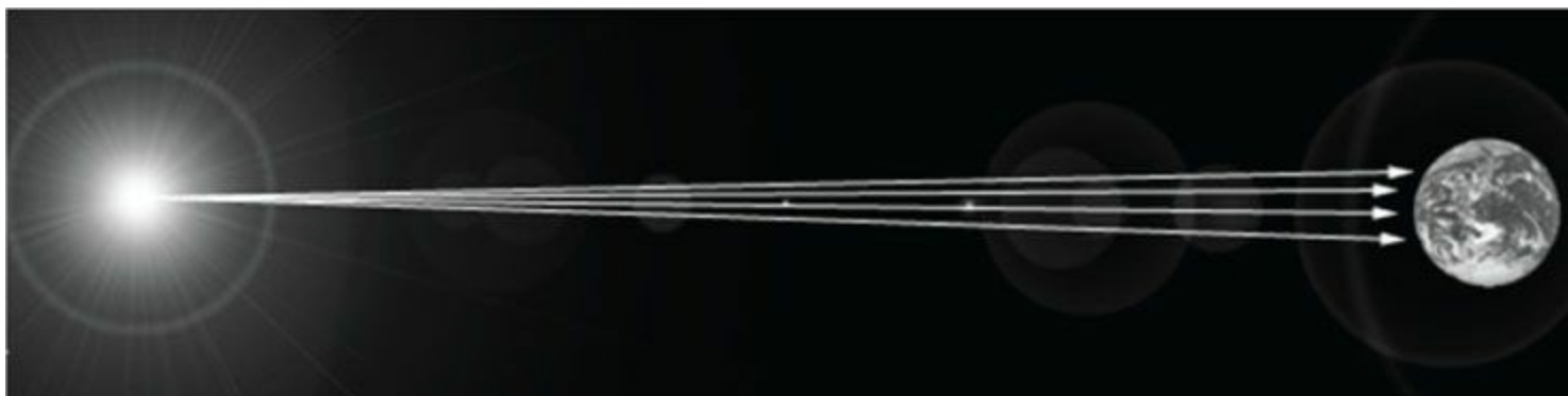
Figure 7.18. The figure is not drawn to scale, but if you select a small surface area on the Earth, the light rays striking that area are approximately parallel.
