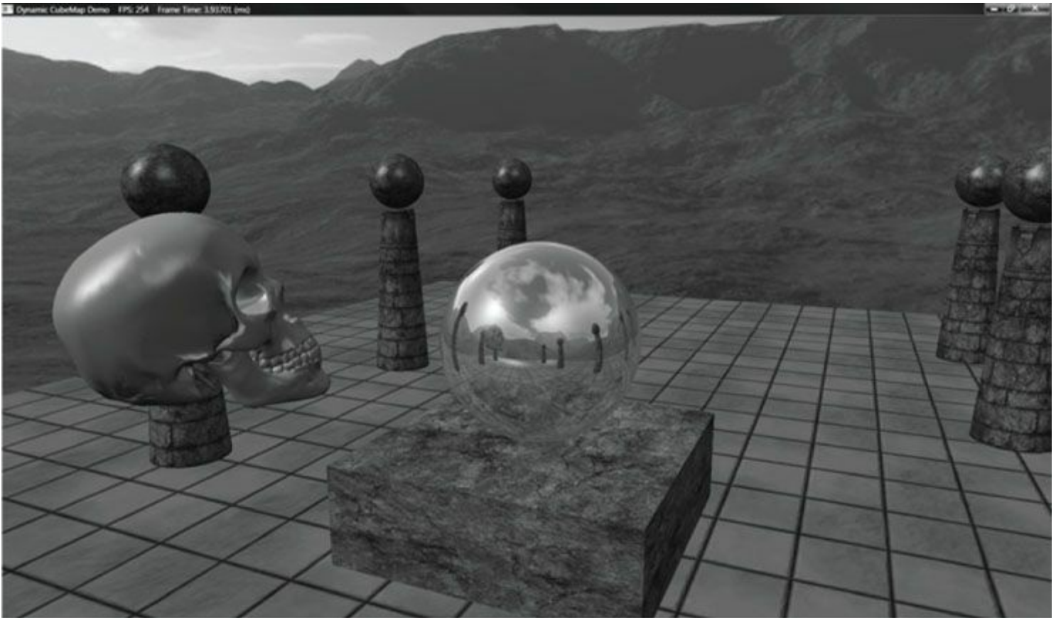
Figure 17.10. Screenshot of the “Dynamic CubeMap” demo showing off dynamic reflections. The skull orbits the center sphere, and its reflection in the sphere animates accordingly. Moreover, because we are drawing the cube maps ourselves, we can model the reflections of the local objects as well, such as the columns, spheres, and floor.
