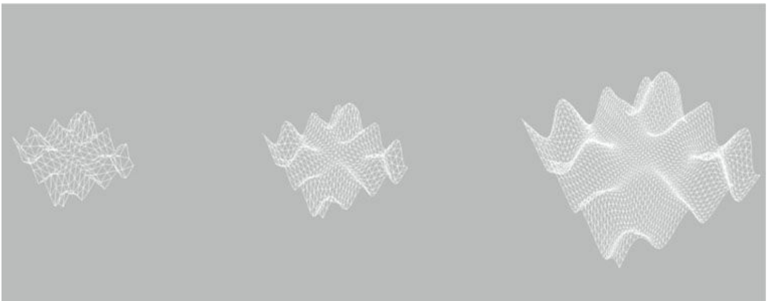
Figure 13.5. The mesh is tessellated more as the distance to the eye decreases.
