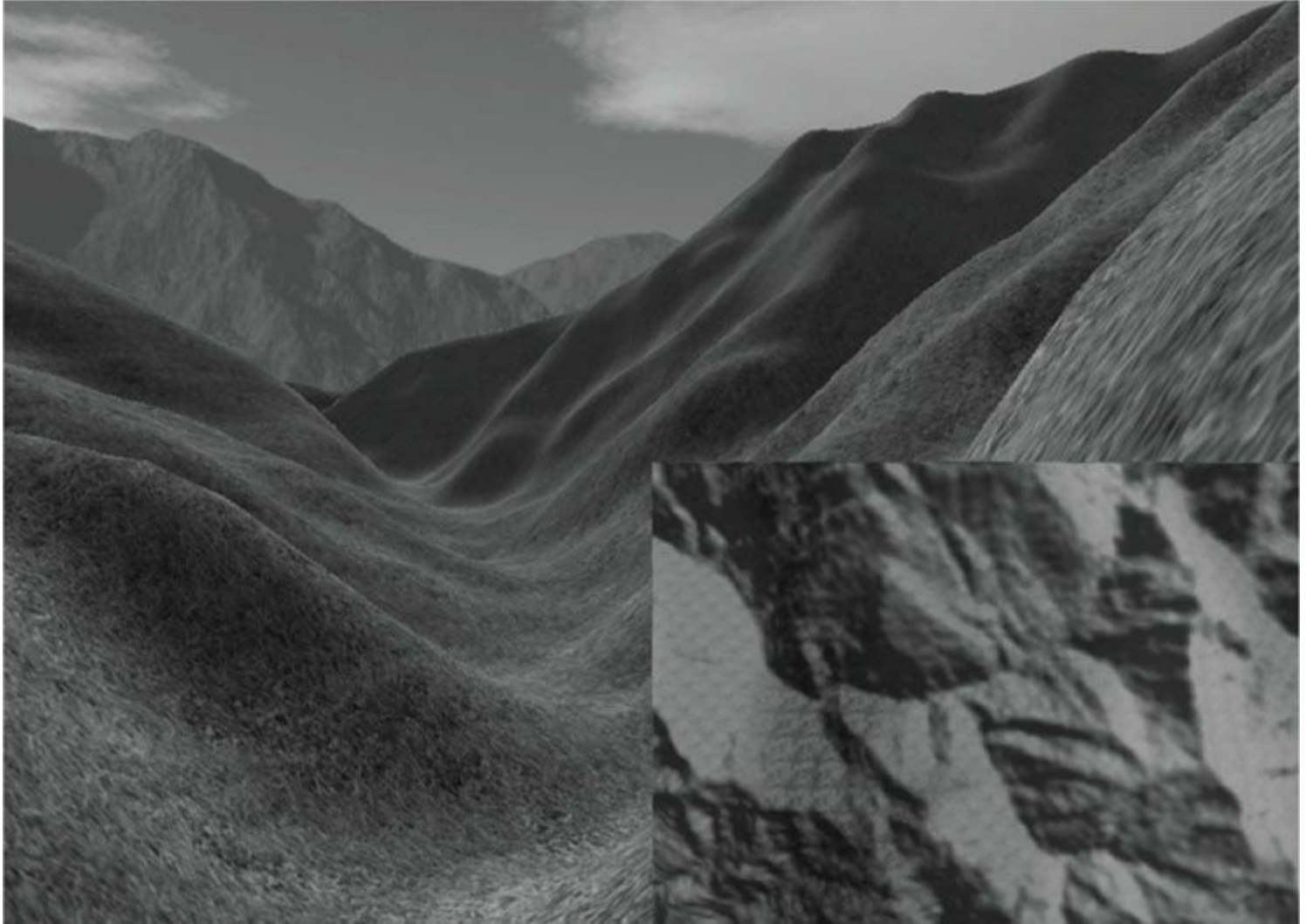
Figure 12.7. A camera is placed above the player from a bird’s eye view and renders the scene into an off-screen texture. When we draw the scene from the player’s eye to the back buffer, we map the texture onto a quad in the bottom-right corner of the screen to display the radar map.
