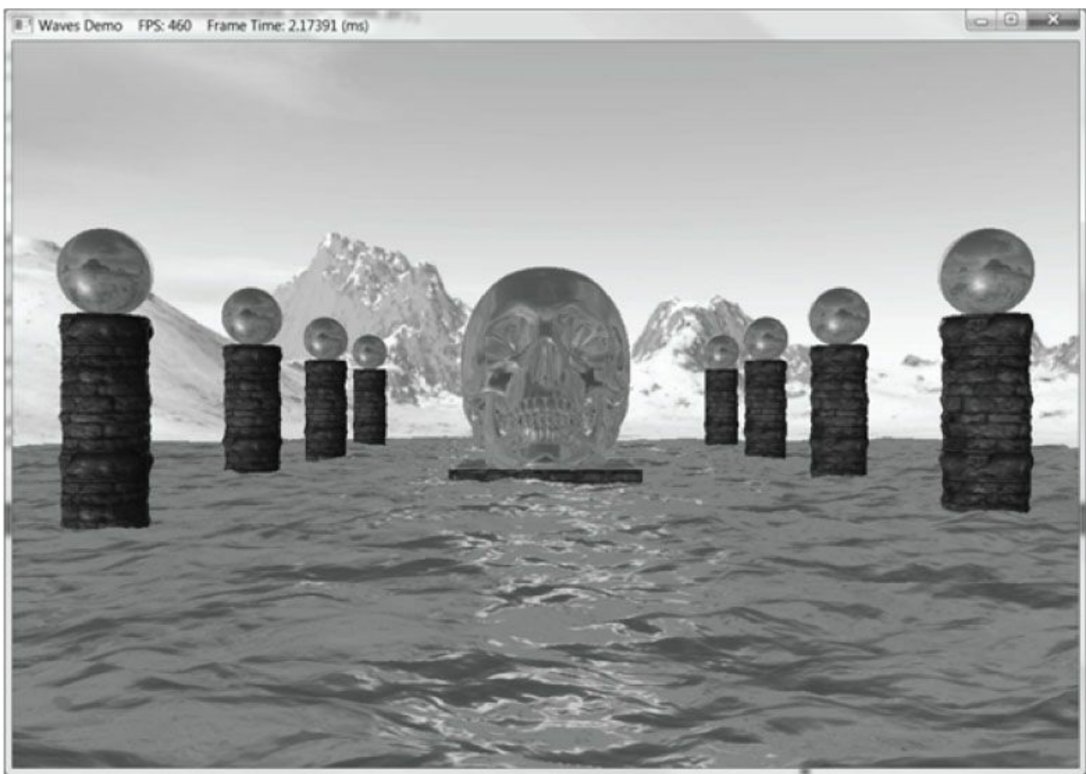
Figure 18.11. Ocean waves modeled with heightmaps, normal maps, and environment mapping.
