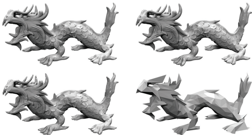
Figure 7.2. Decimation of the dragon mesh consisting of 577,512 triangles (top left) to a simplified version with 10% (top right), 1% (bottom left), and 0.1% (bottom right) of the original triangle count. (Model courtesy of the Stanford Computer Graphics Laboratory.)
